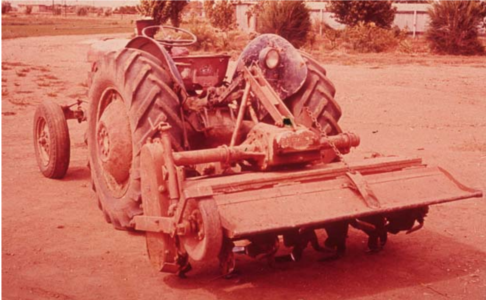
Tractor Used in Glasshouse – the three point linkage rotary hoe was the main tillage implement.
