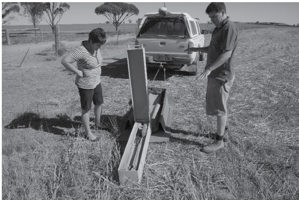
Figure 1 Peter Treloar explains EM38 mapping to Dot Brace. The EM38 unit is attached to the back of a 4WD.
