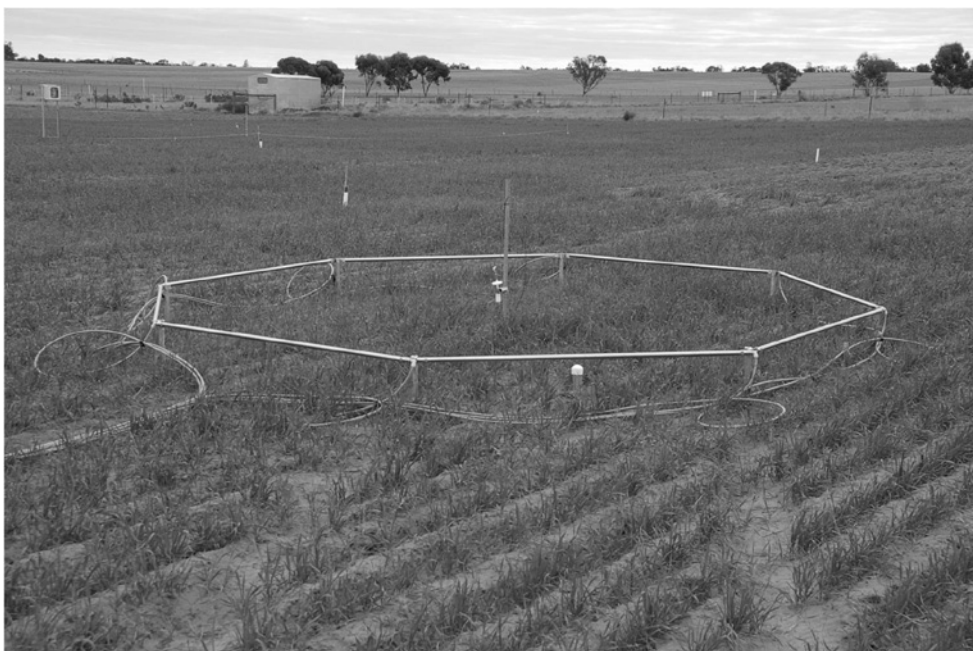
Figure 2 One of the eight free-air carbon dioxide enrichment rings in the field at Walpeup, Victoria. Eight normal plot areas well spaced from these rings were used as comparisons.
