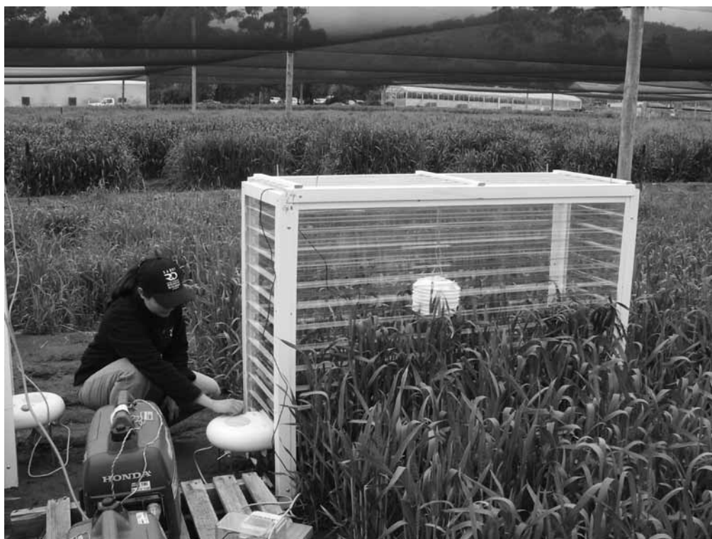
Figure 2 Chamber set up in the field over two rows of wheat, showing a heater at the bottom and TinyTag in a Stevenson screen hanging at canopy height within the chamber
