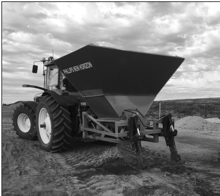
Figure 1. Philips New Horizon machine used to mix slurry and inject manures into the subsoil.
