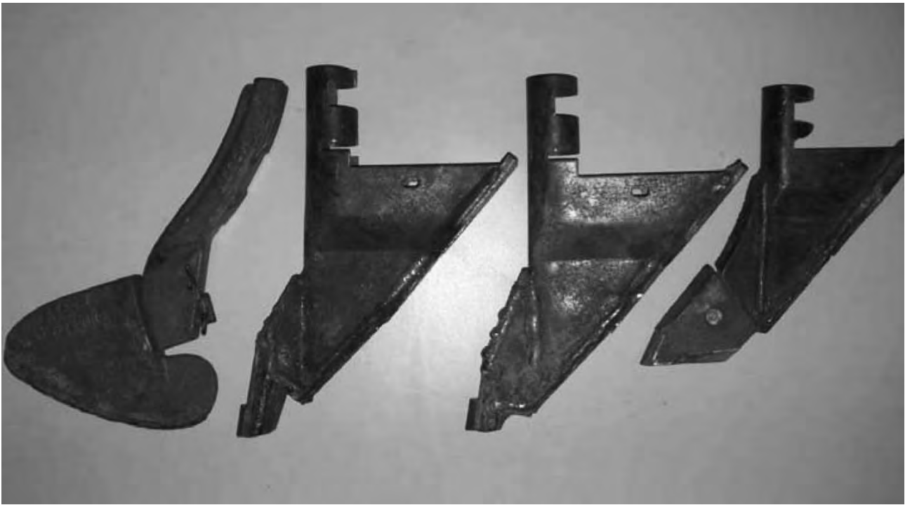
Figure 1 Left to right: Rock Hopper, Atom-Jet Rhizo, Atom-Jet, Bourgault front delivery point
