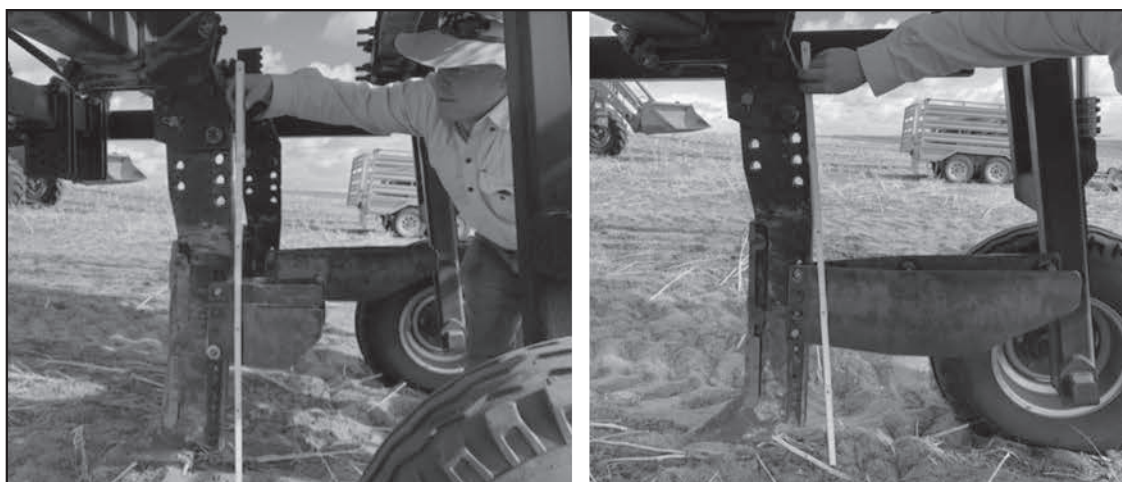
Figure 2. Deep ripper tine with short (250 mm) inclusion plates (left) and long (600 mm) inclusion plates (right).
