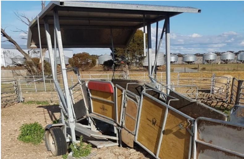
Fig. 4. A Combi Clamp, together with weigh bars, scale head and stick reader, is used to manually draft out hoggets to keep on as breeders, with selections based on individual wool and body weight records.
