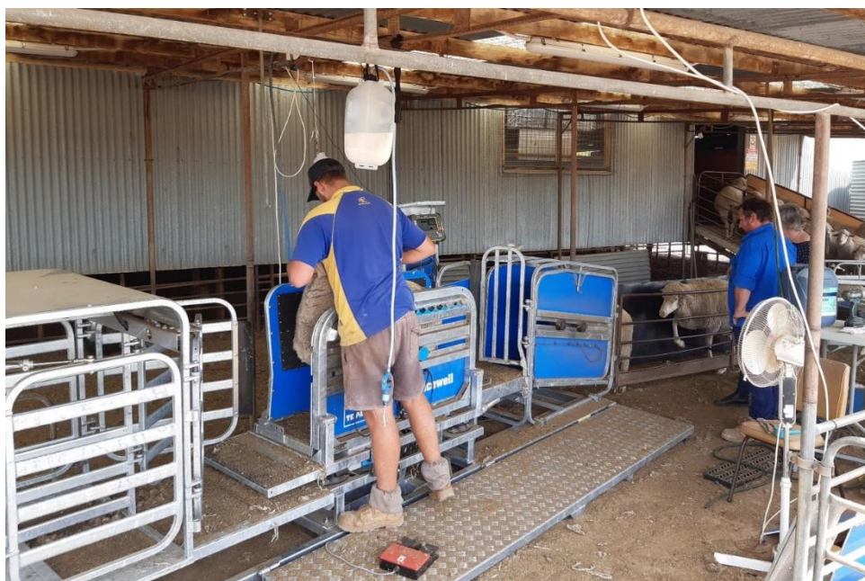
Fig. 1. All animal health treatments at Lampata are conducted through a combined animal handler/autodrafter, allowing frequent recording of weights against eID and reducing manual labour
