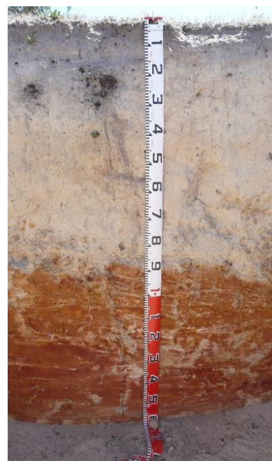
Photo of the soil profile at the Cadgee site, showing a shallow A1 horizon of grey sand, overlying a very deep infertile, acidic, bleached white sand, with B horizon clay generally intercepted below 90 cm.
