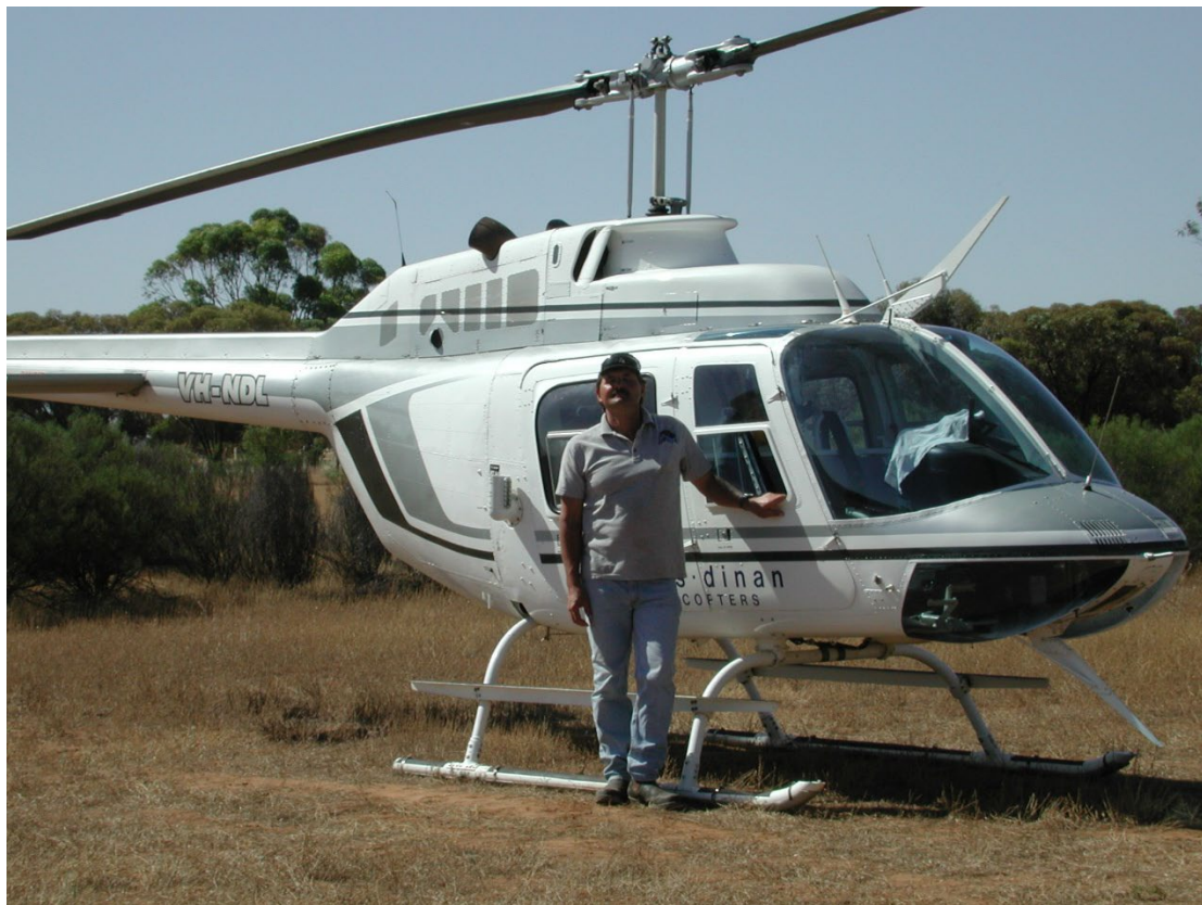
Figure 9: Treva Hebbermann, field worker, and the helicopter from Norris Dinan used in 2010. This Bell JetRanger chopper complies with the guidelines by being turbine powered and fitted with cable cutting devices that protrude from the top and floor of the cabin.
