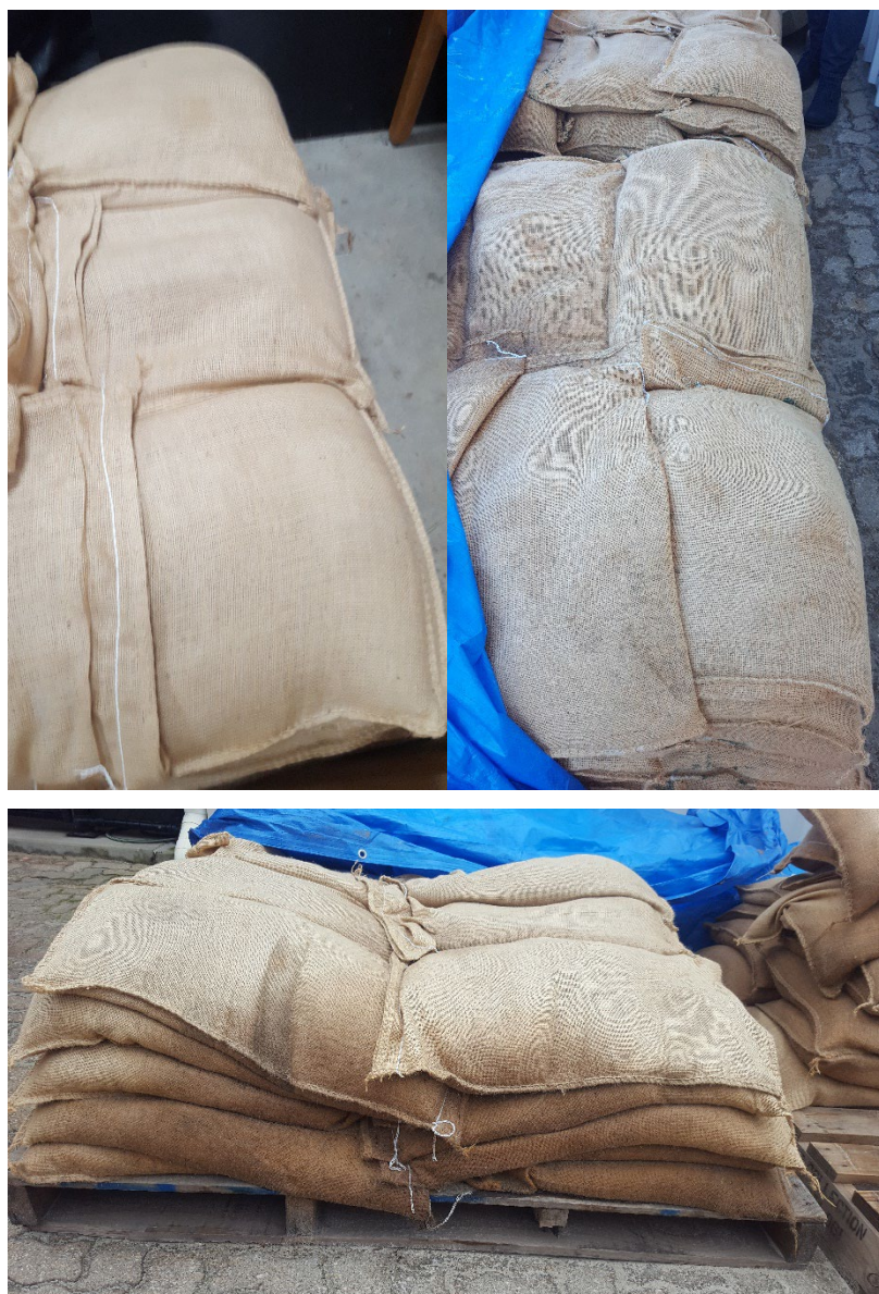
Figure 7-1: Examples of bags located inside (top left), outside under a tarp (top right) and outside exposed to the elements (bottom).
