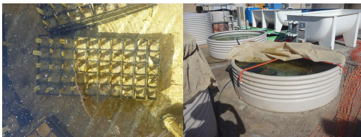
Figure 6-1: Posidonia tank experiment set-up showing a tray of 50 pots planted with Posidonia seedlings (left) and a tank used for holding the seedlings (right).
