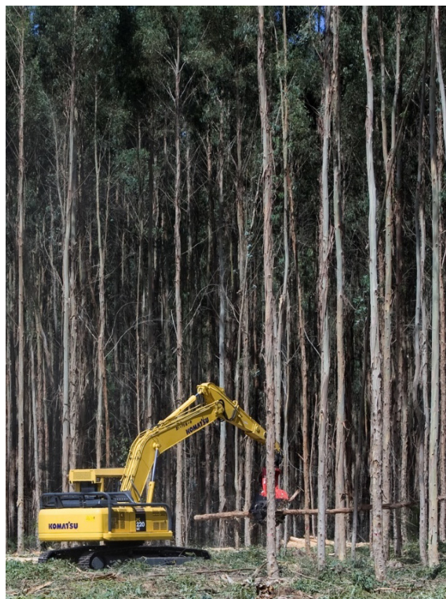
Figure 2. Mechanical timber harvester processing Tasmanian bluegum (Source: PIRSA)
