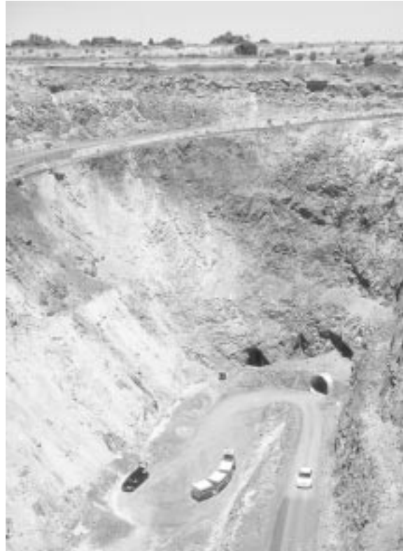
Wheal Hughes open cut and mine portal. (Photo 46546)
