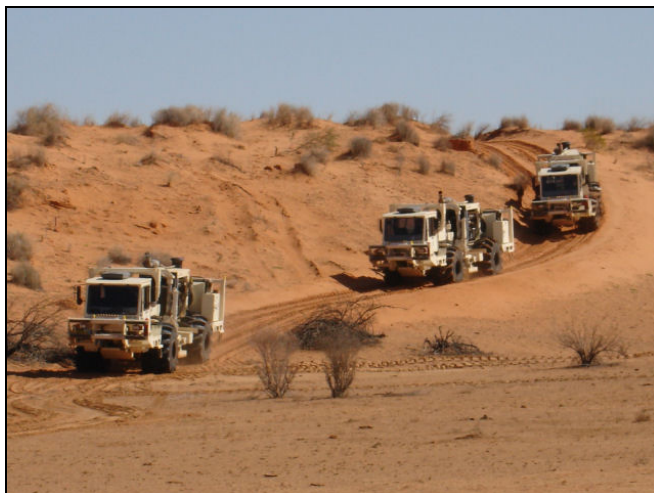
Plate 2: Vibrator trucks traversing a seismic line
