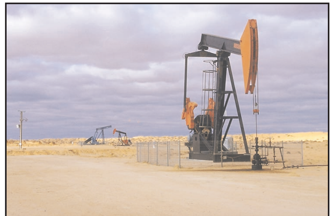
Beam pumps producing oil, Merrimelia Field. (Photo 45016)
