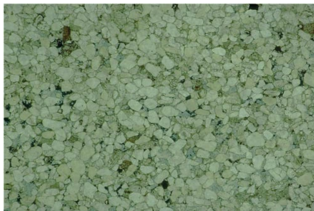
Relief Sandstone at 178.9 m in Observatory Hill 1. Porosity, coloured blue, is ~20%. Plane polarised light; field of view is 6.8 mm. (Photo 44385)
