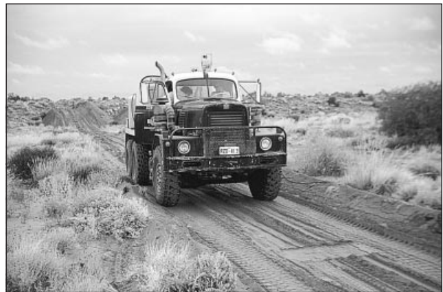
One of the earliest operations in Australia to use vibrators for seismic surveys was in the Simpson Desert in May 1974. (Photo 43831)
