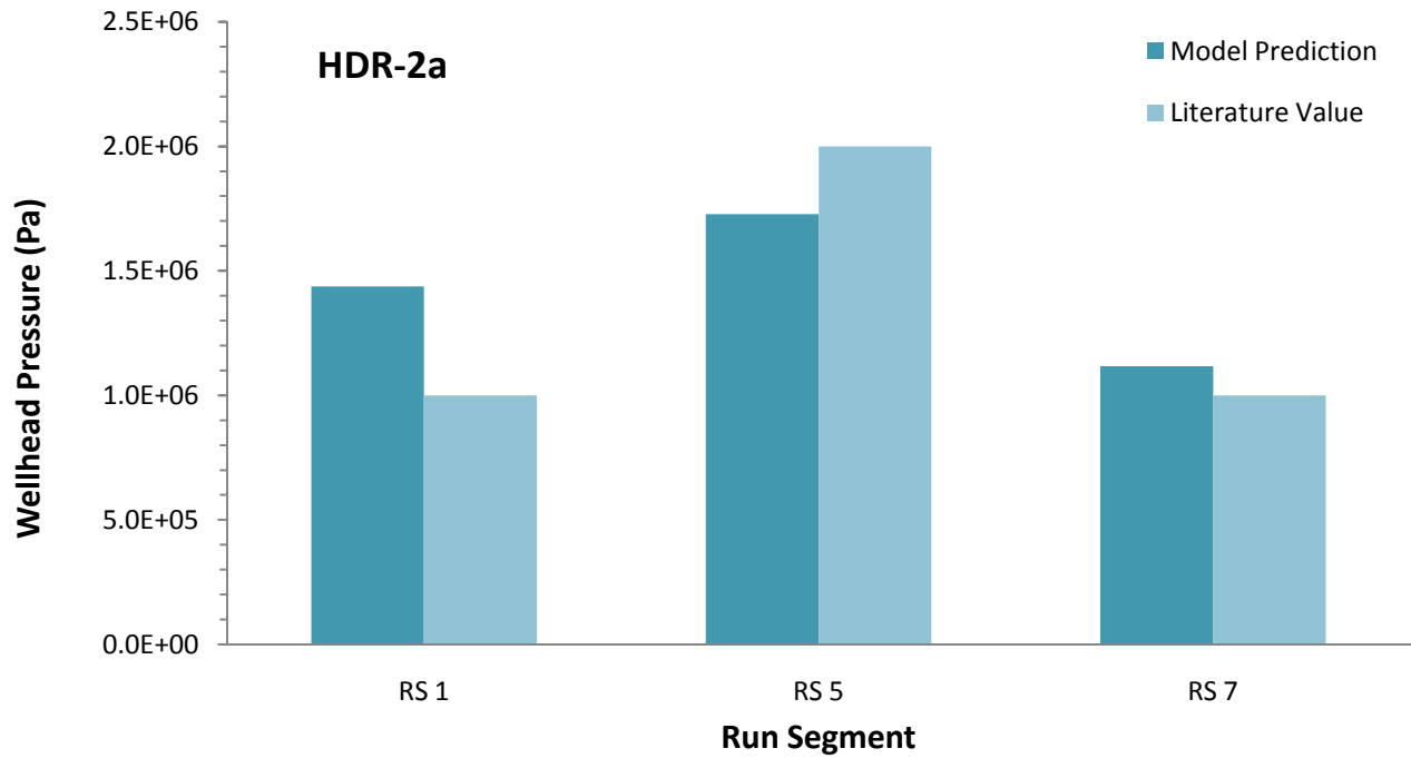
Figure 32 Comparison of model predicted and literature values of wellhead pressure for HDR-2.
