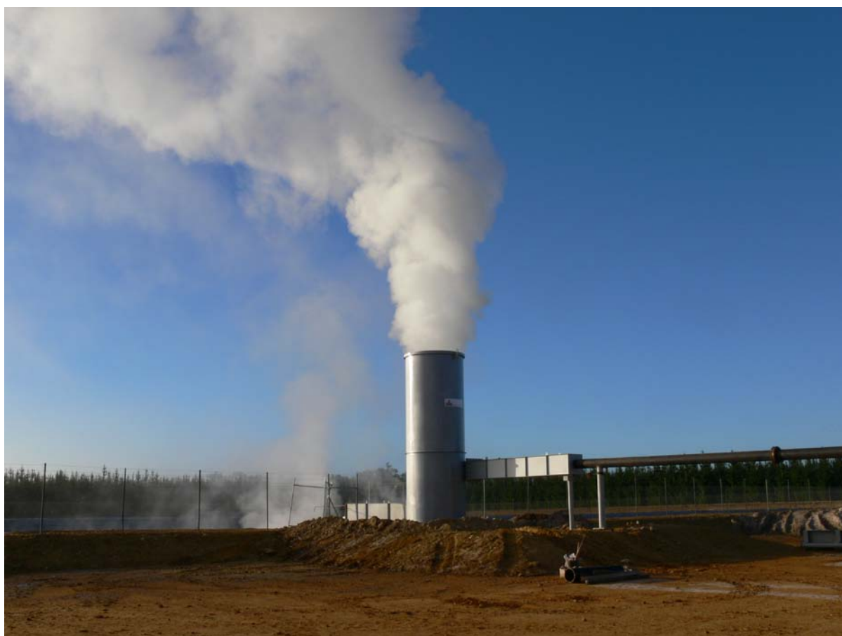
Flow test at Panax Geothermal's Salamander 1 well, the first deep well drilled at the Penola Hot Sedimentary Aquifer Project in the south east of South Australia. Photo courtesy of Panax Geothermal.
