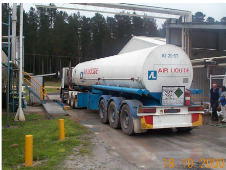
Plate 4: CO 2 transport tanker in loading area.
