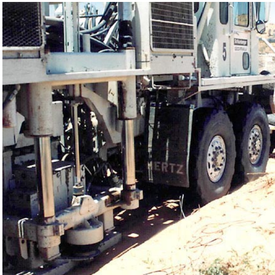
Plate 3 Vibrator pad. (photo 047924)
