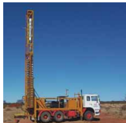
Investigator Mark 10 auger drill. (Photo 049376)
